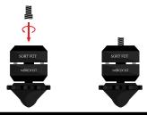
WHILE HOLDING THE TOP OF THE SORT FÜT BODY, THREAD ONTO SPEAKER UNTIL TIGHT
