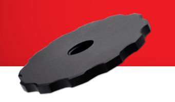
The Sort Lock is a locking wheel upgrade that allows you to fix the adjustments that you have made to your Sort Füt units. It should be fitted to the Sort Füt before installation. This is done by removing the adjustable finial dome and screwing the locking wheel onto the threaded post.
